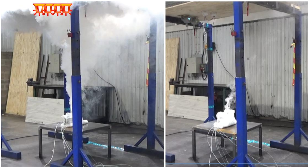
Figure 8. Right: Smoke covering the point-type detectors in Test 1. Left: The less vigorous production of gas/smoke in Test 2.
