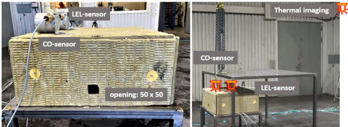
Figure 3. Left: Photo of the hood with the CO and LEL sensors. The 50 mm × 50 mm opening was there to allow a controlled release of gases. Right: The hood and the shielding covering the battery cell.
