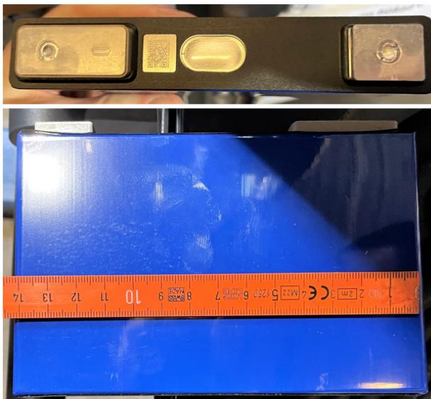
Figure 1. Photo of one of the battery cells used in the tests.
