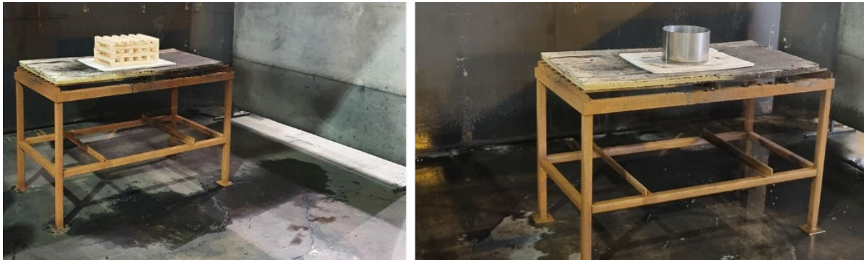
Figure 31: Smaller wood crib fire source (left) and smaller heptane fire source (right) for mechanical ventilation tests.
