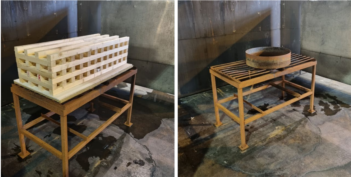
Figure 23: Larger wood crib fire source (left) and larger heptane fire source (right) for natural ventilation tests.
