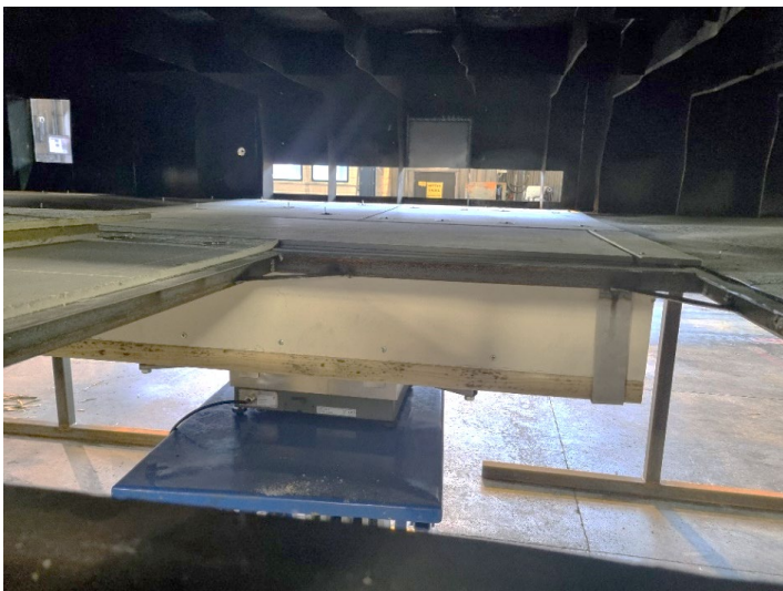
Figure 35: Weighing platform from inside the model.
