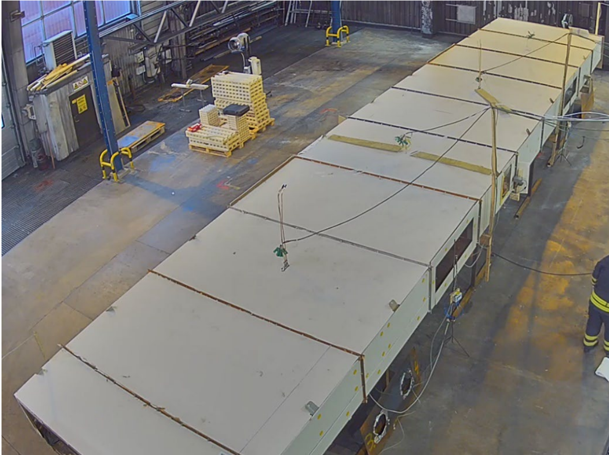
Figure 17: The model of the ro-ro space was built up in the fire hall in Borås. Section 1 is in the bottom left of the figure, and Section 10 is in the top right of the figure.
