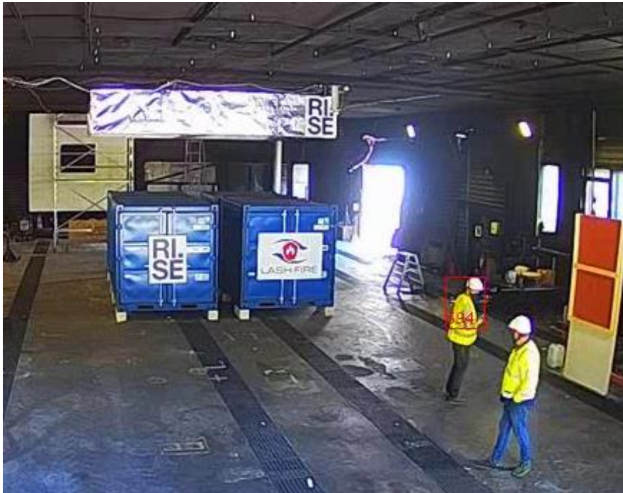
Figure 32: Example nuisance alarm from the video fire detection algorithm that has misinterpreted the moving reflective jacket of a person as a growing flame and has marked it with a red rectangle.
