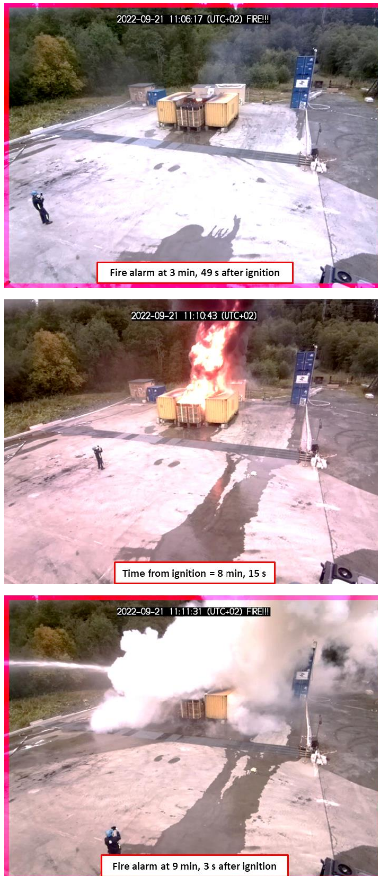
Figure 49. Video images from the built-in camera of the triple-IR flame wavelength detector during a fire suppression test scenario with a 300-s waiting time after flames were visible. Top figure shows the first fire alarm. Middle figure shows moments before fire suppression. Bottom figure shows another fire alarm immediately after fire suppression.
