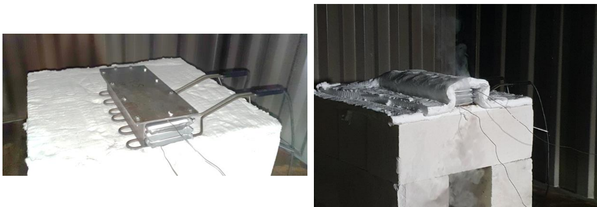
Figure 23: Overheating three lithium-ion battery cells in a steel enclosure with electric heating elements. The steel box was open in the front. Insulation was placed on top of the box during tests to get a more uniform heating of all three cells.
