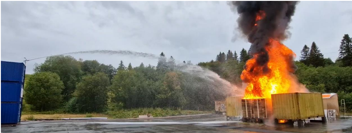
Figure 44: Photo showing the activation of a fire monitor during a late-suppression scenario (300-s waiting time)
