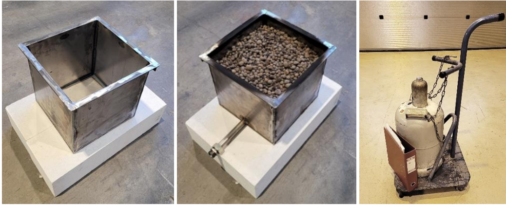
Figure 36: Tray for the heptane pool fire (left) and the equivalent gas burner (middle) used with a propane bottle (right).
