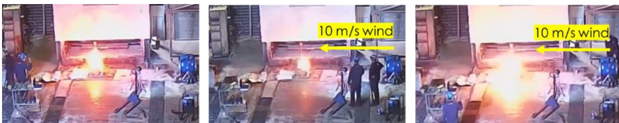
Figure 41: Wind effects visible in footage snapshots of a flame captured by a camera at 27.1 m horizontal distance and 10 m height: the wind causes the fire to appear smaller sometimes (middle photo) and bigger at some other times (right photo) due to the image saturation and flame reflections from nearby surfaces.
