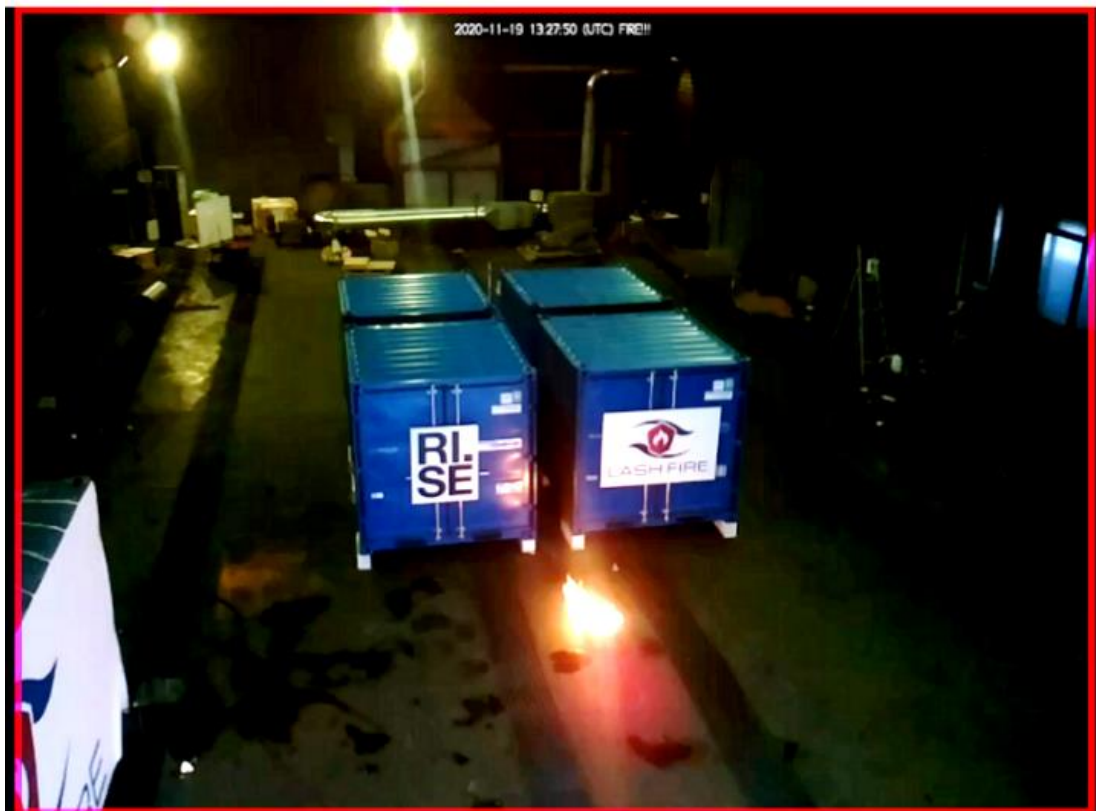
Figure 24: Video image from the built-in camera of a triple-IR flame wavelength detector triggered by a flame during a LASH FIRE test. When the alarm is activated, the frame around the image turns red and the text "FIRE" is shown on the upper part.
