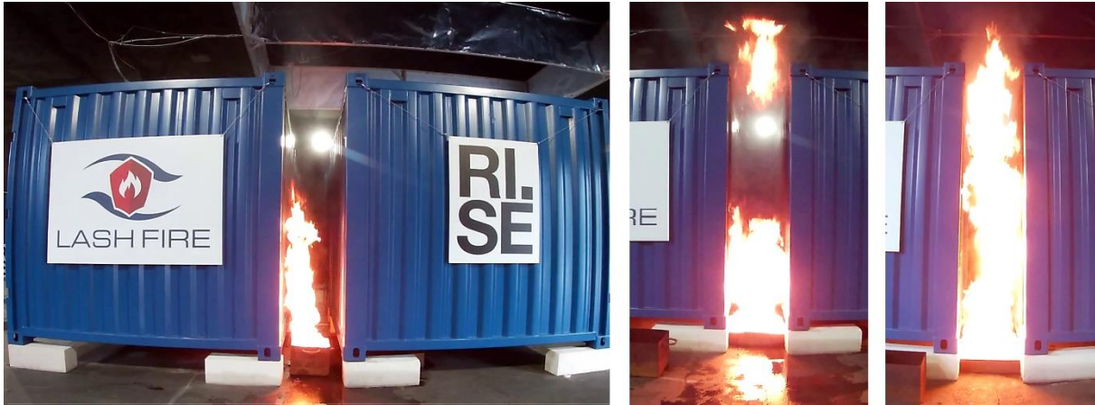
Figure 22: Maximum extension of the flame lengths for the three heptane pan fires of 30 x 30 cm (left), 50 x 50 cm (middle) and 60 x 60 cm (right).
