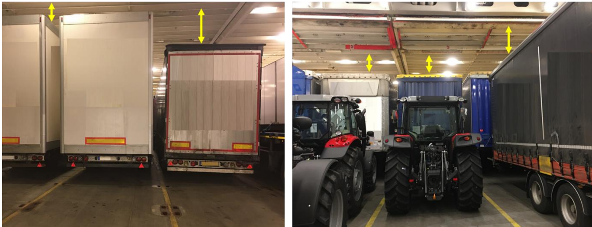
Figure 9: Typical free space above cargo items (height shown with yellow arrows) which limit the field of view of cameras installed on the deckhead of ro-ro spaces. The tallest items in the field of view will define the extent of free height available.
