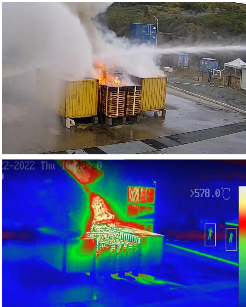
Figure 46: A snapshot from a regular video camera (top) and a snapshot from a thermal imaging camera (bottom) during a fire suppression experiment with two fire monitors in the late fire suppression scenario (300-s waiting time). The persons in the background have been highlighted manually to illustrate the usefulness of this information from the thermal camera.
