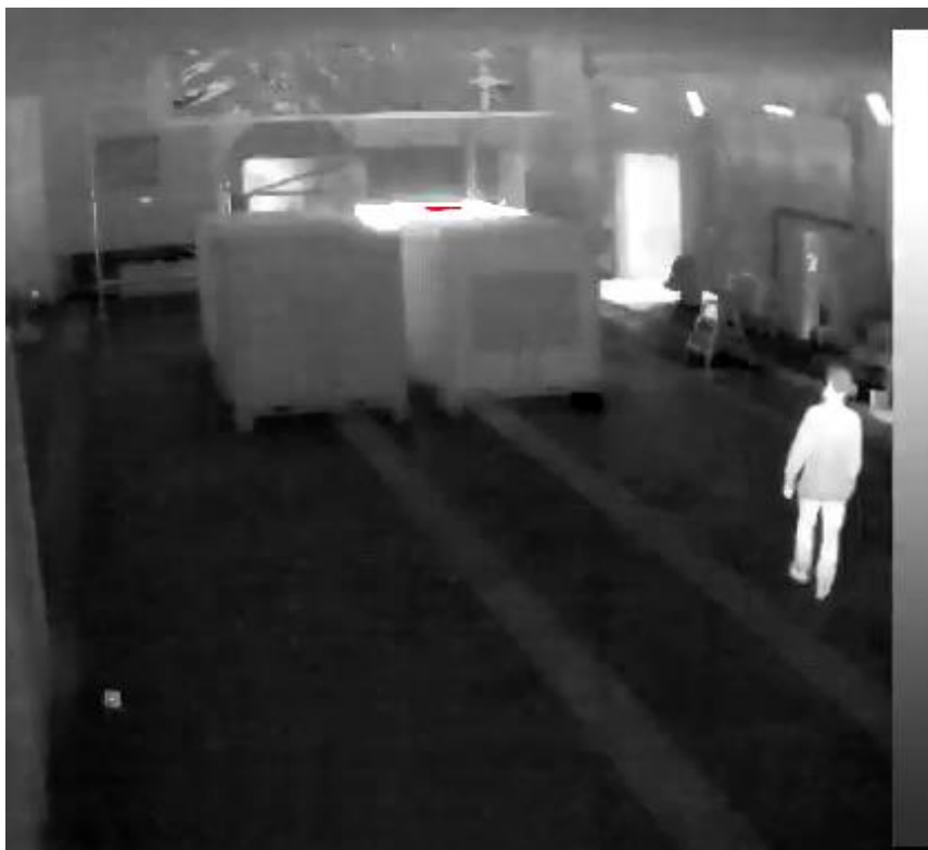
Figure 29: A fire inside a closed container detected by a thermal imaging detection system using an infrared camera (test 13 in Table 7). The hot roof of the container is marked with a red colour by the detection software to highlight the region of alarm.
