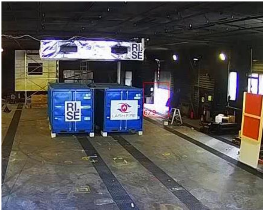
Figure 33: Example nuisance alarm from the detection algorithm due to the gate of the test hall rolling up to let light in, which has been recognised falsely as a growing flame (outlined using a red rectangle).
