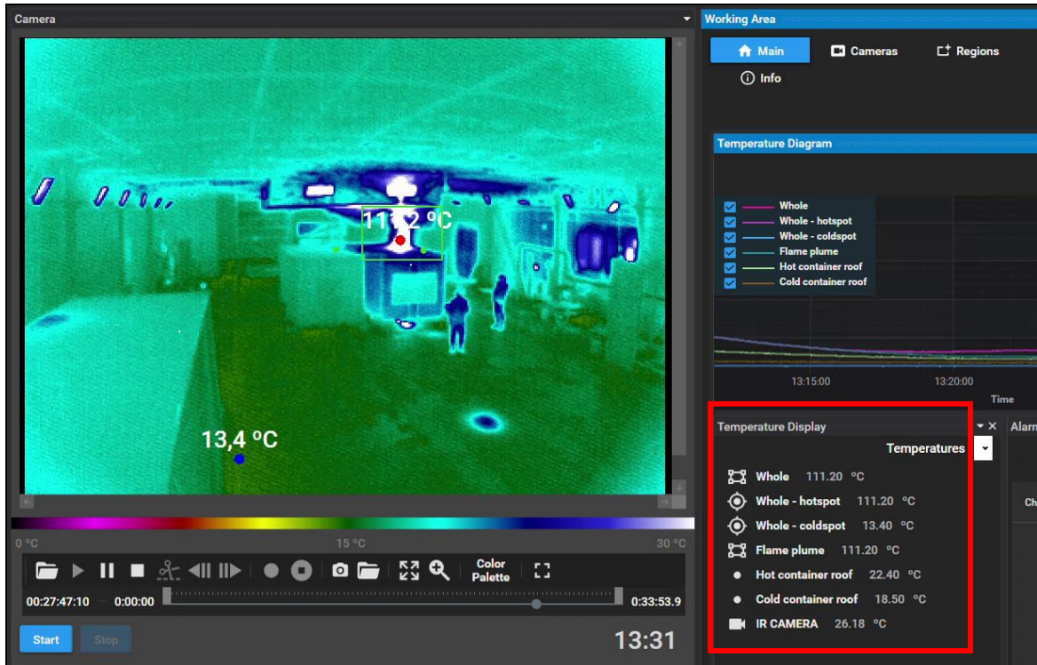
Figure 26: Screenshot from the software of thermal camera IR2 during test 19 (described in Table 8). Temperatures from selected hot areas are measured (see red rectangle) and recorded over time (see graph in Figure 28).
