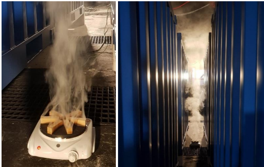
Figure 21: Beechwood sticks on a hot plate generating light grey smoke without flames.
