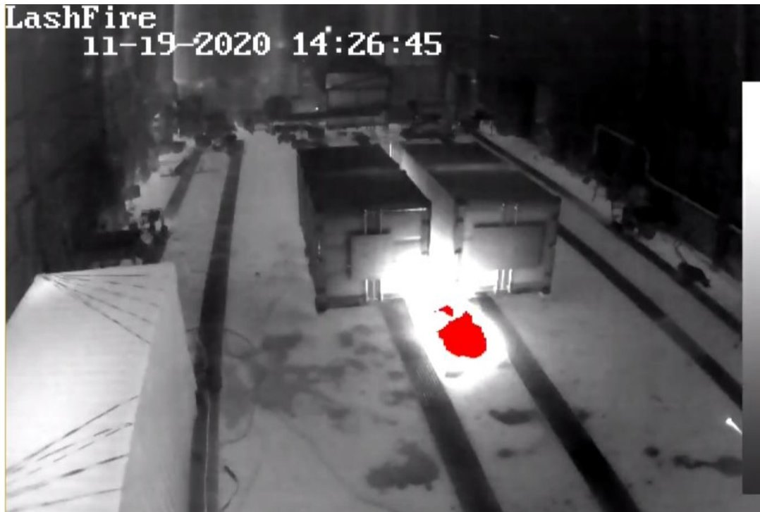
Figure 25: Snapshot from the footage of a thermal imaging camera captured during a demonstration test. The high temperature area of the fire is marked with red, clearly drawing attention to the hot spot (see regular image in Figure 24).
