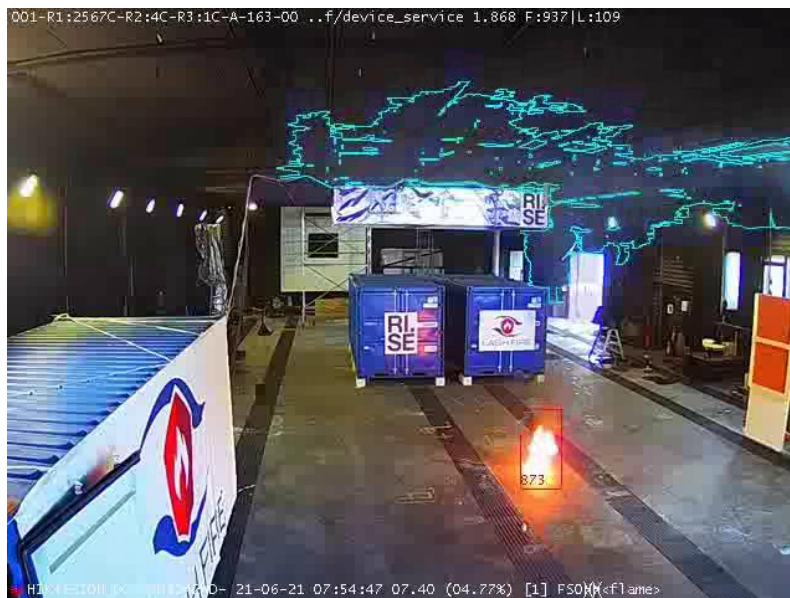
Figure 31: Image from a CCTV camera processed in real time by the video fire detection software during a demonstration test. The flame on the floor and the smoke along the ceiling are marked by the software with red and blue outlines, respectively.
