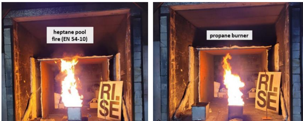
Figure 36: Tray for the heptane pool fire (left) and the equivalent gas burner (middle) used with a propane bottle (right).
