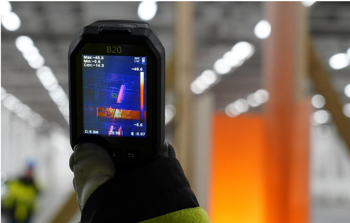
Figure 51: Handheld thermal camera showing temperatures along the deckhead during fire test scenario D shown in Figure 46.
