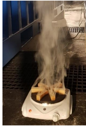
Figure 17: Beechwood sticks on a hot plate generating light grey smoke without flames.
