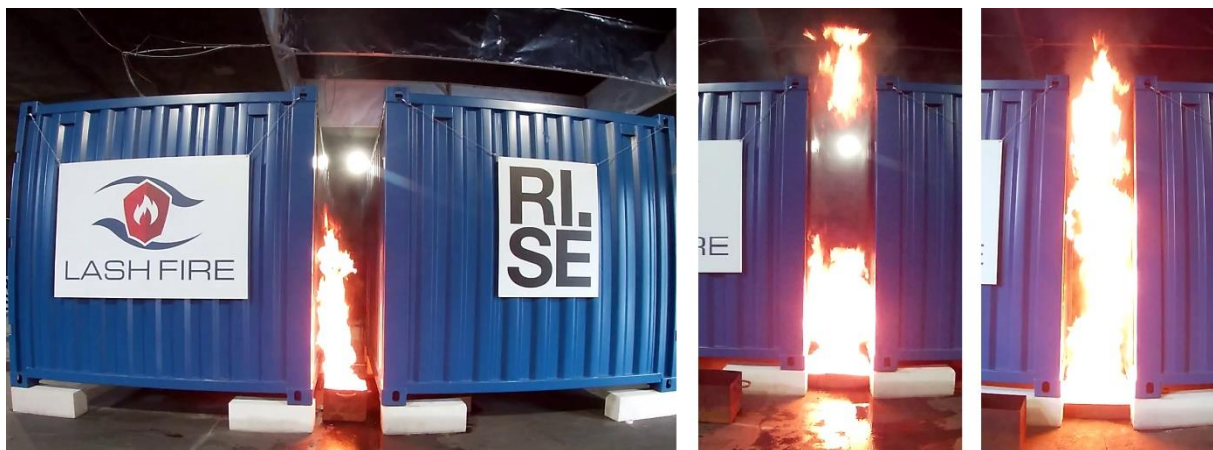
Figure 18: Maximum extension of the flame lengths for the three heptane pan fires of 30 x 30 cm (left), 50 x 50 cm (middle) and 60 x 60 cm (right).
