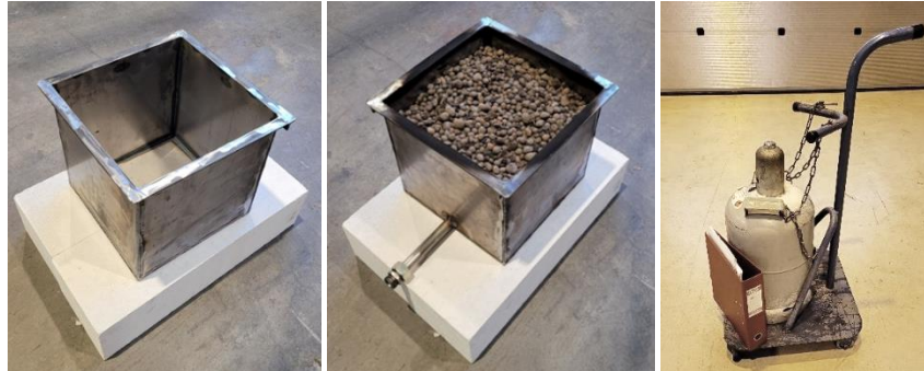
Figure 23: Tray for the heptane pool fire (left) and the equivalent gas burner (middle) used with a propane bottle (right).
