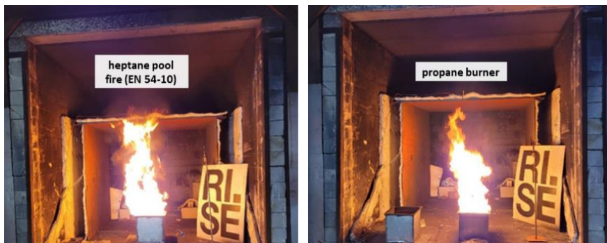
Figure 23: Tray for the heptane pool fire (left) and the equivalent gas burner (middle) used with a propane bottle (right).
