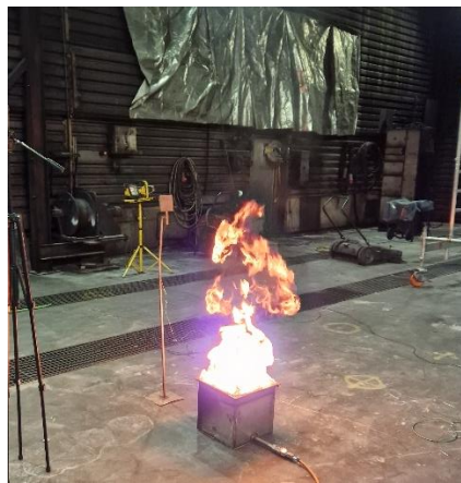
Figure 27: Reference fire test conducted with no panels.
