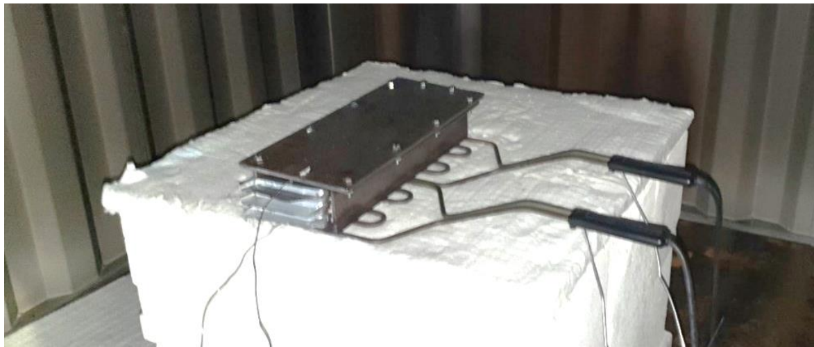
Figure 19: Overheating three lithium-ion battery cells in a steel enclosure with electric heating elements. The steel box was open in the front. Insulation was placed on top of the box during tests to get a more uniform heating of all three cells.
