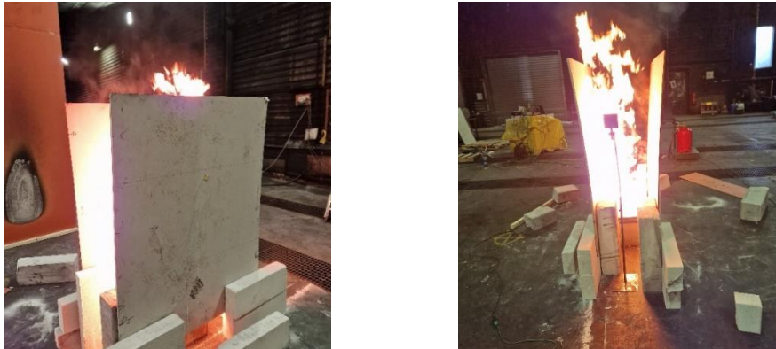
Figure 26: Test setup for fire test with gypsum panels simulating the effect of two cars placed near the ignition source.
