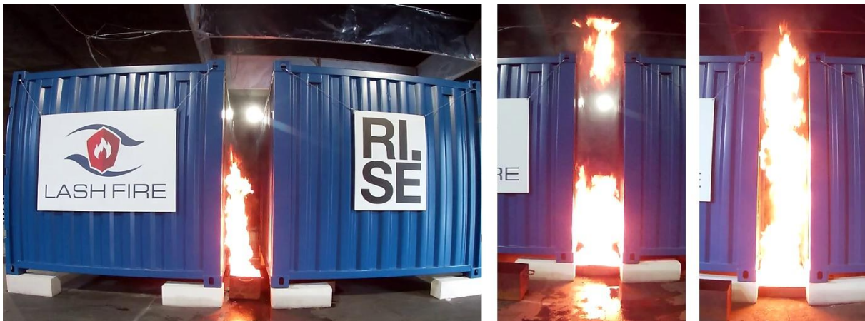
Figure 16: Maximum extension of the flame lengths for the three heptane pan fires of 30 x 30 cm (left), 50 x 50 cm (middle) and 60 x 60 cm (right).
