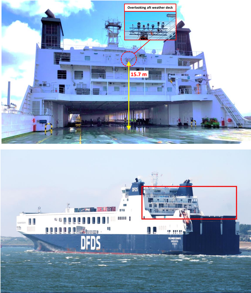
Figure 34: LASH FIRE detectors fixed on deck 11 of Hollandia Seaways with a view to deck 7, i.e., the aft weather deck (highlighted in the bottom figure from [51]). Table 13 lists the detectors, which were on board from Feb 2022 until July 2023.
