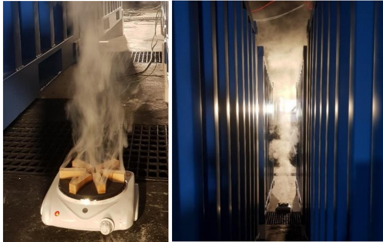
Figure 15: Beechwood sticks on a hot plate generating light grey smoke without flames (as described in EN 54-29 [41]).
