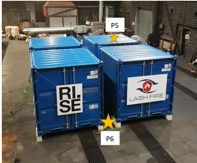
Figure 12: The test containers from the viewpoint of the detectors on the wall. Fire positions P5 and P6 were directly visible to the detectors, while the other fire positions were shielded between or inside the containers (see Figure 13).
