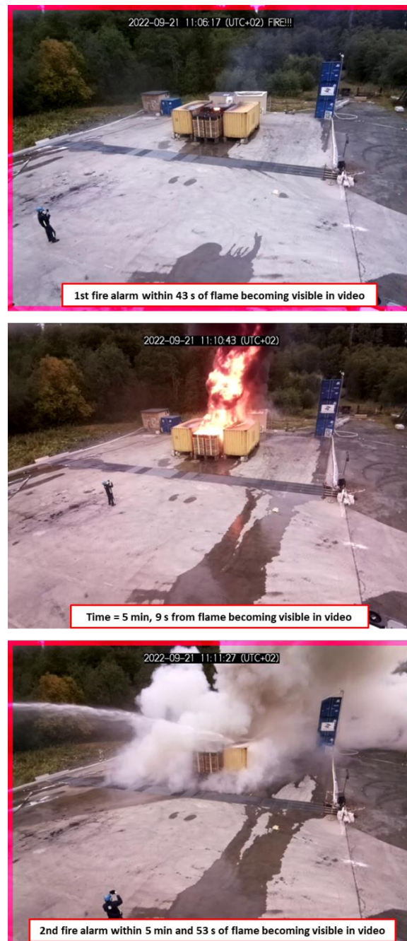
Figure 32. Video images from the built-in camera of the triple-IR flame wavelength detector during test 6 described in Table 12 (late suppression with fire monitors A and C shown in Figure 29). Top figure shows the first fire alarm. Middle figure shows moments before the activation of fire monitors. Bottom figure shows the second fire alarm after the activation of fire monitors.
