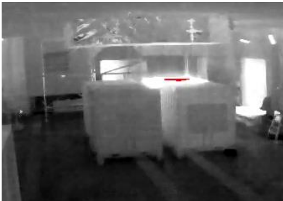
Figure 17: A fire inside a closed container detected by a thermal imaging detection system during test 13 (Table 9). This image is captured by thermal camera IR1, showing the hot roof of the container with a red colour. This fire was not detected by the flame wavelength detectors as no flames were visible outside the container.
