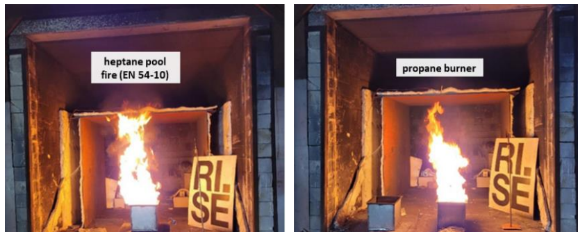
Figure 21: Tray for the heptane pool fire (left) and the equivalent gas burner (middle) used with a propane bottle (right).
