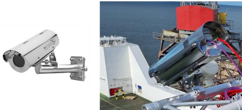
Figure 5: Example thermal imaging (infrared) camera installed on board Hollandia Seaways for LASH FIRE evaluations.
