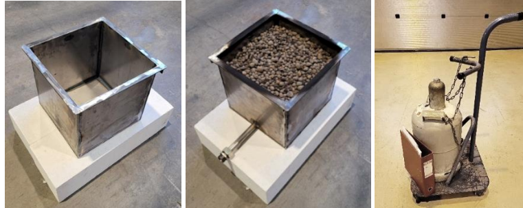
Figure 21: Tray for the heptane pool fire (left) and the equivalent gas burner (middle) used with a propane bottle (right).
