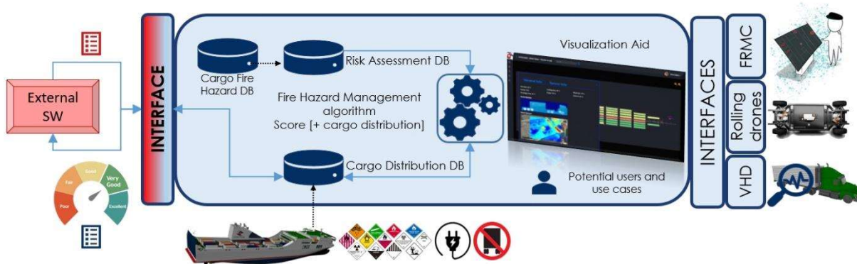
Figure 2 - Software components of the Stowage Planning Tool
