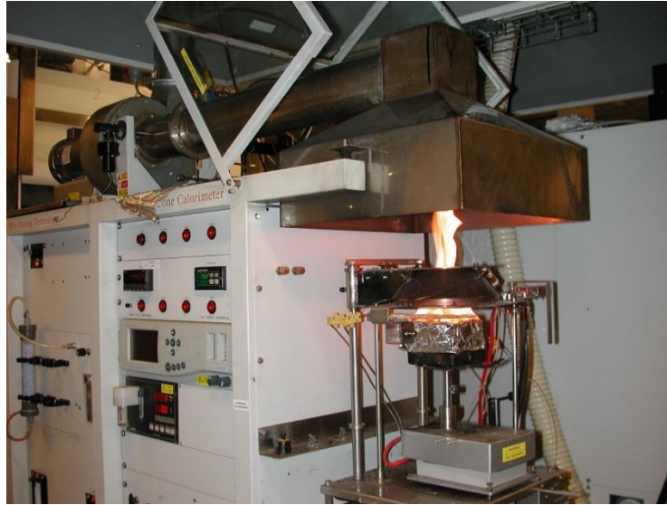
Figure 5 The cone calorimeter equipment according to ISO 5660-1.
