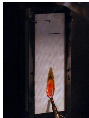
Figure 11 Surface exposure of a material according to EN ISO 11925-2
