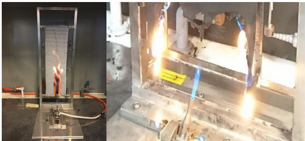
Figure 10 Test equipment for test of vertical burning rate according to ECE Regulation 118, Annex 8.
