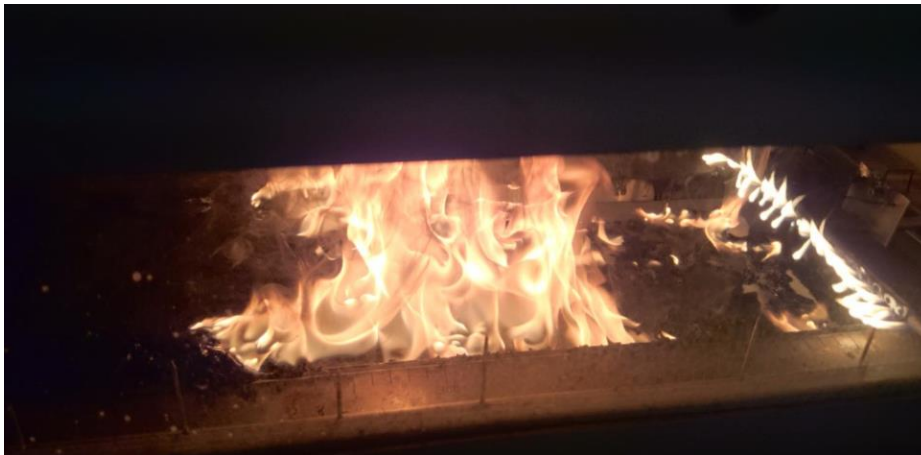
Figure 8 Floor covering during fire test according to EN ISO 9239-1.
