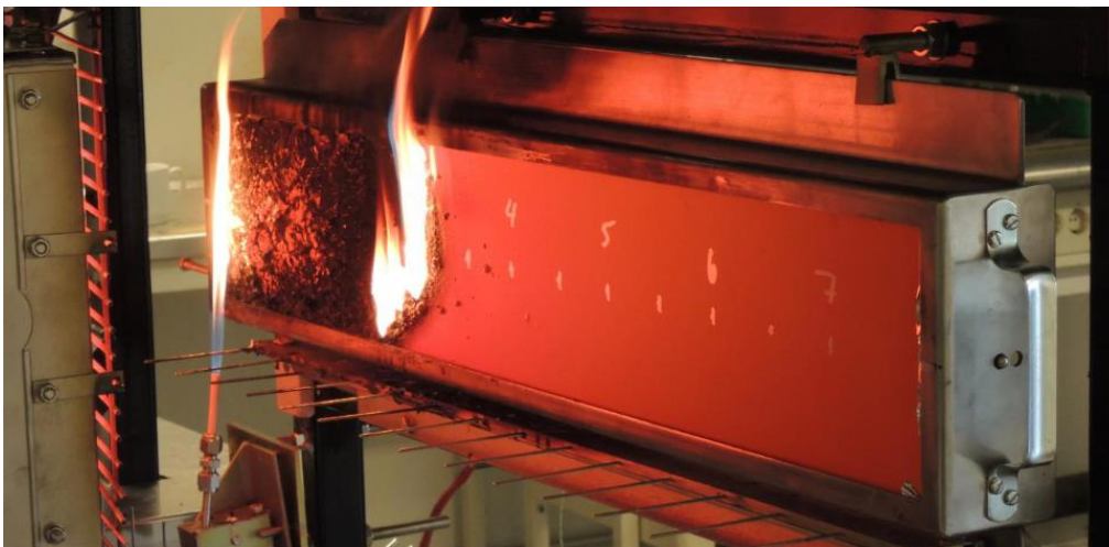
Figure 4 Specimen during fire test with the spread of flame equipment.
