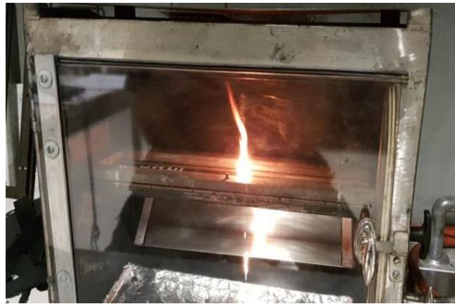
Figure 9 Fire test of material in the equipment for horizontal burning rate, FMVSS 302.
