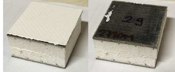
Sample 29 – PET/Basalt/Polyester/Intumescent coating
