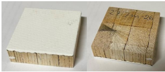
Sample 26 – Balsa/Glass/PFA/Intumescent coating
