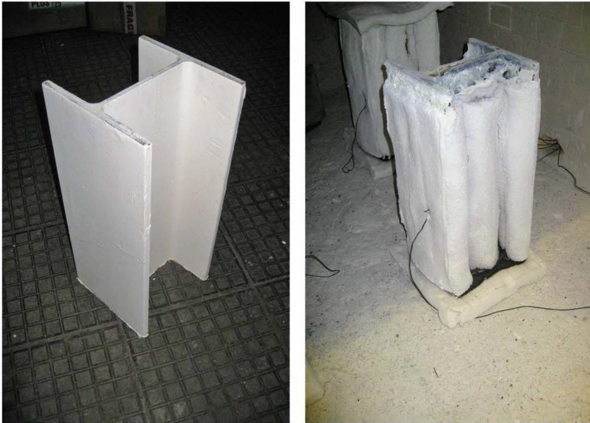
Figure 18. Steel beam coated with intumescent coating – under normal temperature and swelled during the fire
