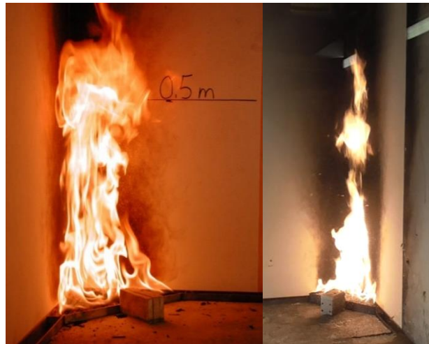
Figure 6 Schematic drawing of the SBI test set-up. A corner in the room is built of the material to be tested with a 30 kW burner in the corner.
