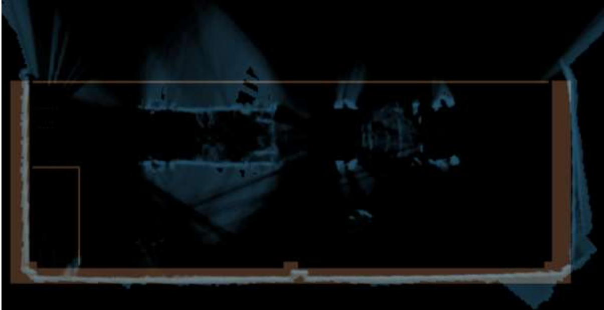
Figure 28 LiDAR used for SLAM on global map.
