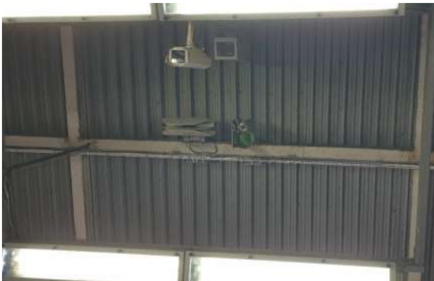
Figure 18 LiDAR and LWIR for left side of the vehicle. (RISE)
