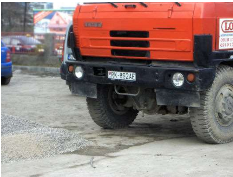
Figure 43 Failure to detect vehicle by OpenALPR. Image modified from [19].
