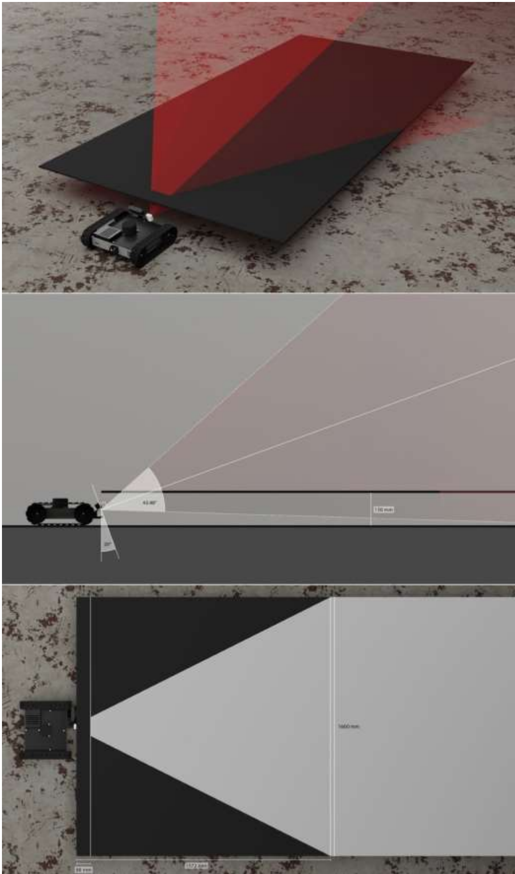
Figure 28 Coverage of a typical passenger vehicle's battery with the IR camera.
