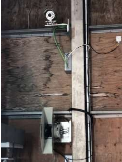
Figure 17 Sensor array including the ambient temperature sensor. (RISE)
