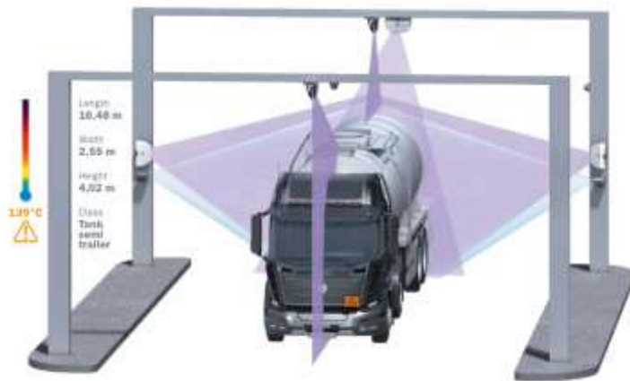
Figure 1 Illustration of the physical installation of a VHD system (SICK)
