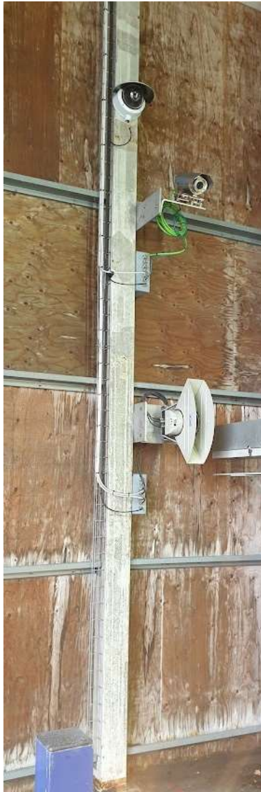
Figure 16 LiDAR and LWIR for right side of the vehicle. (RISE)
