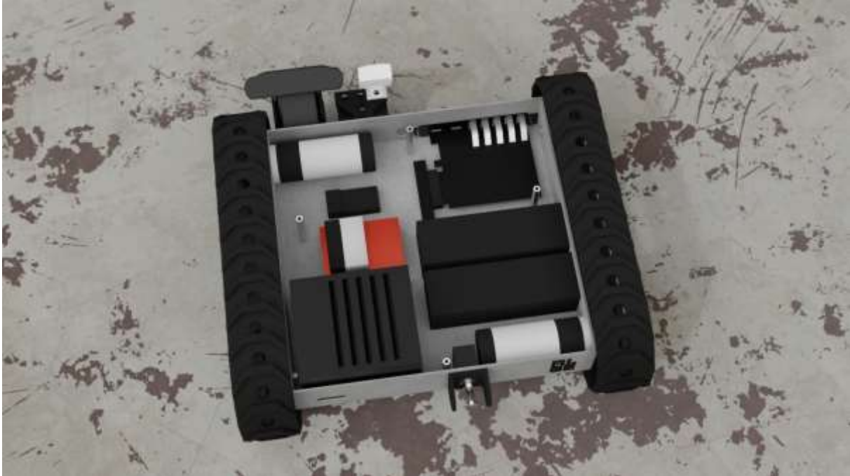
Figure 29 Render of the AGV's final internal component layout.
