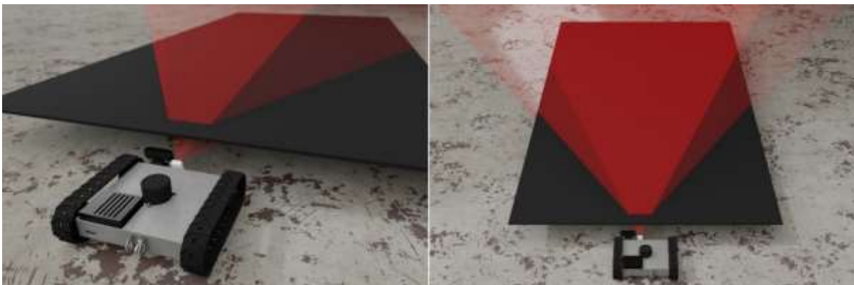
Figure 31 Render of an earlier version of the AGV with a visual depiction of the IR camera's field of view.
