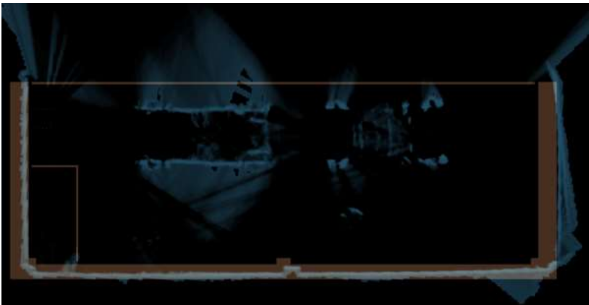
Figure 46 Rotation aligned overlay of SLAM map (blue) and corresponding static environment map (brown). Alignment was carried out with the use of the (combined) global map.
