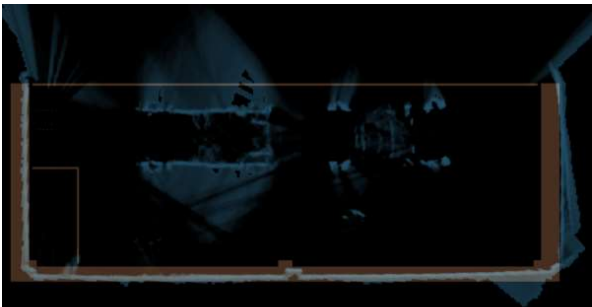
Figure 38. Rotation aligned overlay of SLAM map (blue) and corresponding static environment map (brown). Alignment was carried out with the use of the (combined) global map.
