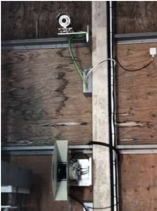
Figure 16 Ambient temperature, LWIR and LiDAR. (STL)
