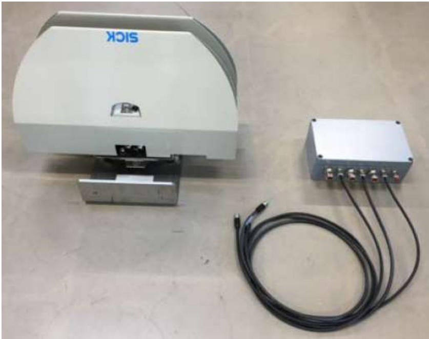
Figure 10 LiDAR with flare protection and junction box. (SICK)
