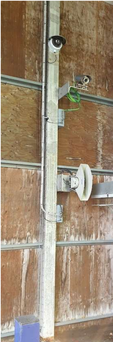
Figure 15 Sensor for profiling and IR scanning the sides. (RISE)
