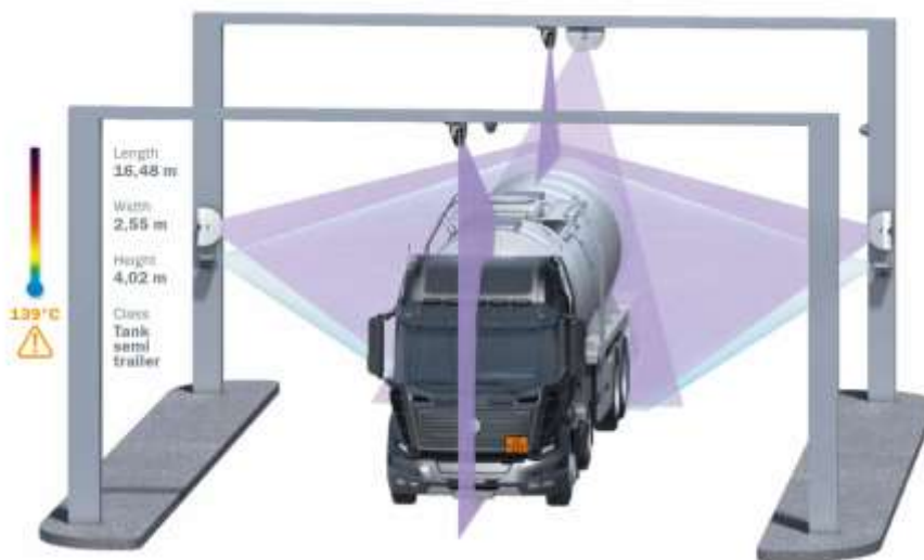
Figure 1 Illustration of the concept of the LASHFIRE VHD sensor portal (SICK)
