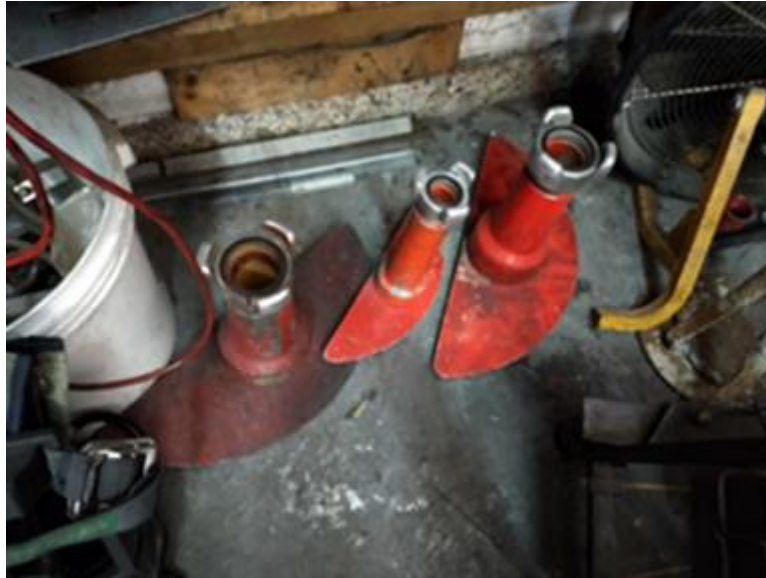
Figure 4 - Water curtain nozzles
