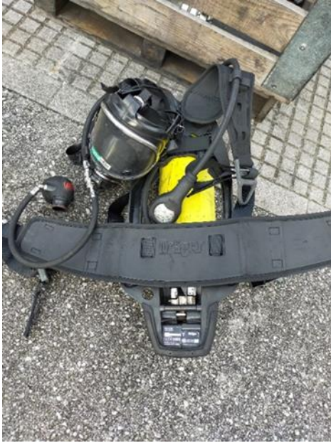
Figure 23. Full BA set with air cylinder, backplate, face mask and demand valve.
