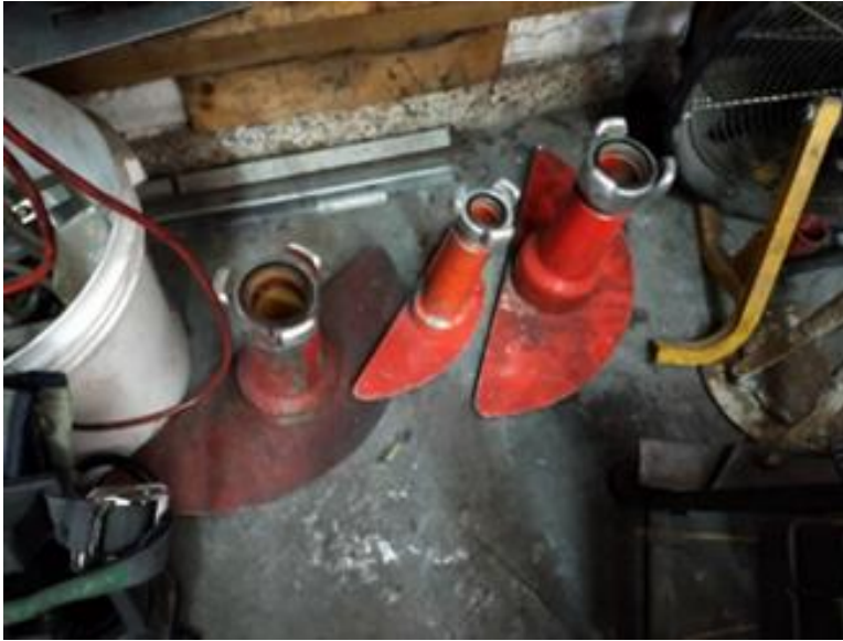
Figure 6. Water curtains. Finally, not used for testing.
