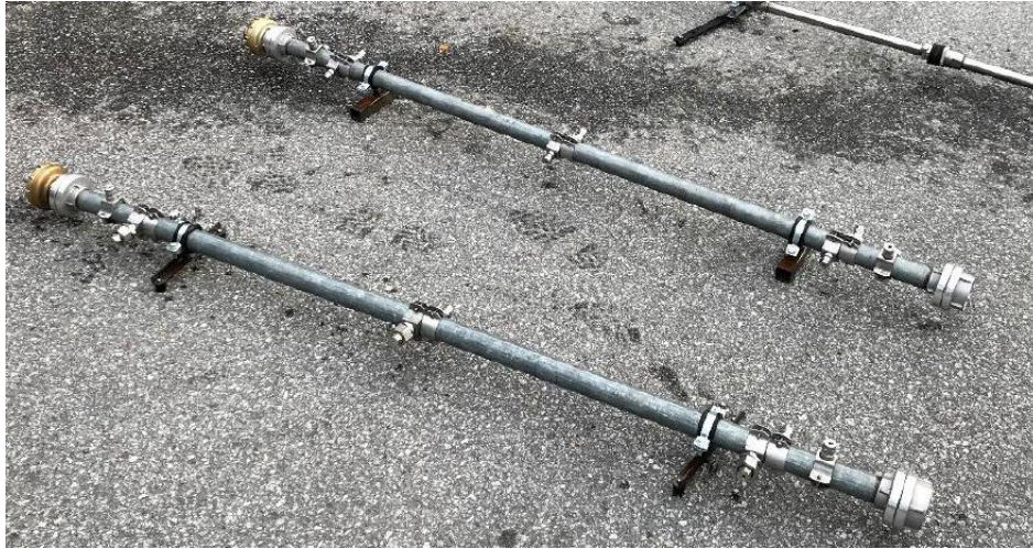
Figure 36: boundary cooling device tested at SAS facilities. (version 1.0)
