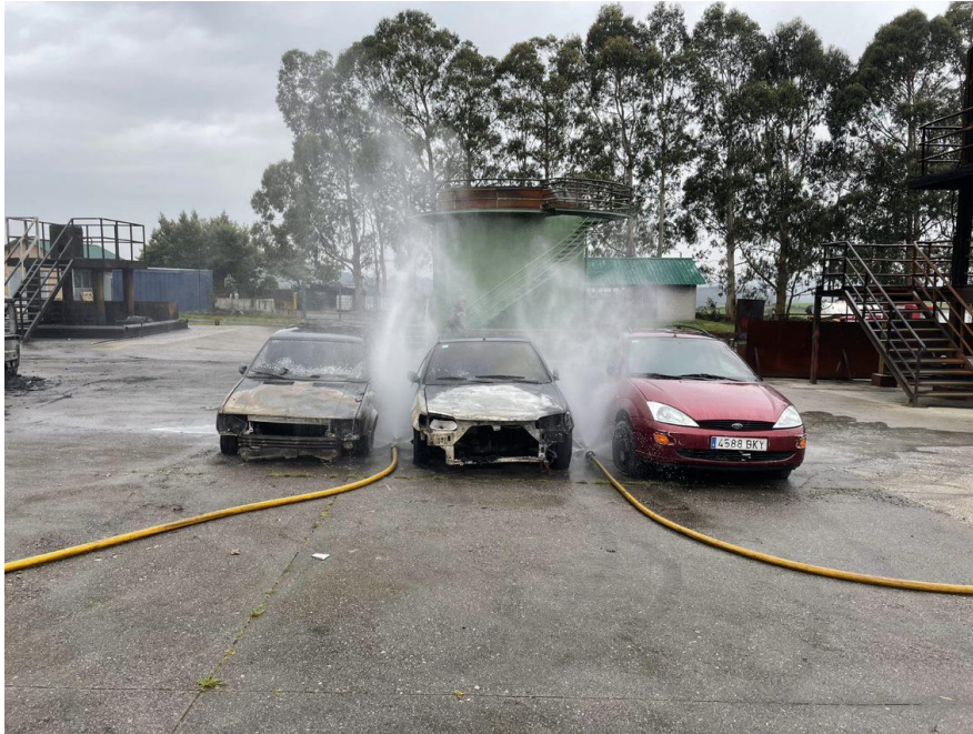
Fig 35. Car's set up for the boundary cooling test.
