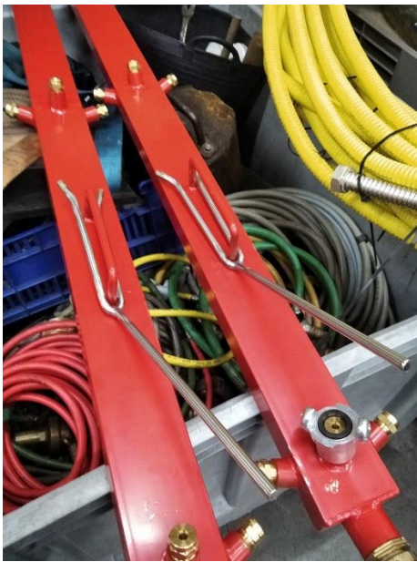
Figure 9. Boundary cooling devices. Version 2.0. Note the hooks attached to a long rod to push the device into position
