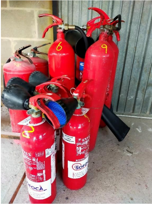
Figure 12. 2 and 5 kg portable CO2 fire extinguishers.
