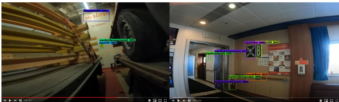
Figure 5 The SMAS platform relies on state-of-the-art deep learning on a datacentre where train the Machine Learning (ML) models that recognize objects particular to vessels. The ML models are then transferred to the Smartphone app.
