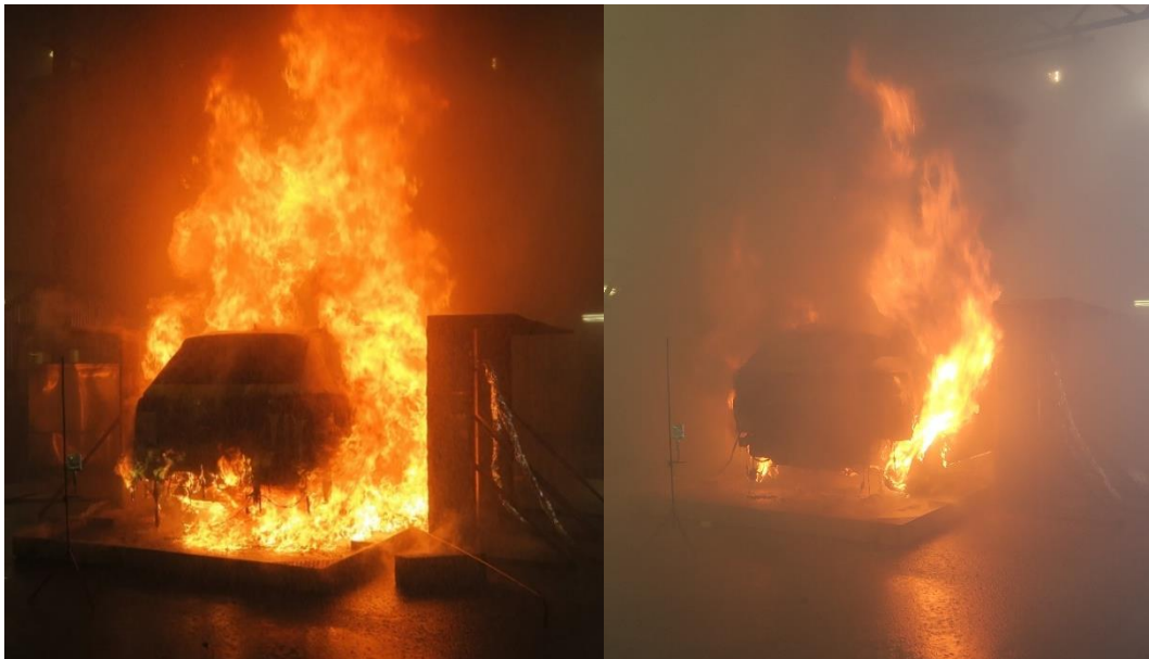
Figure 14. The ICEV1 fire size (left) at the most intense stage at about 03:30 [min:s] as compared BEV1 at the most intense stage at about 19:00 [min:s], viewed from a position in front of and behind the vehicle.
