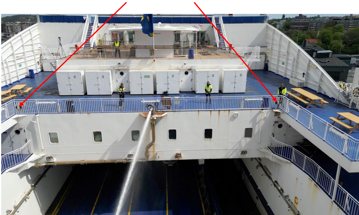
Figure 7. Autonomous fire monitor suppressing a weather deck fire and showing the position of the system's Force 80 fire monitor and its two IR3 flame detectors.
