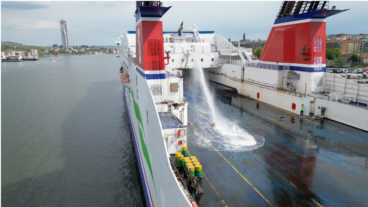
Figure 10. Photo taken during of one of the twelve demonstrations in which the autonomous fire monitor detected, located, and extinguished a propane burner fire onboard the Stena Scandinavica.
