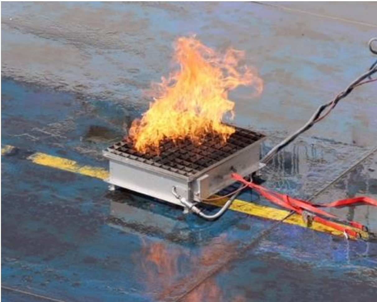
Figure 8. A close-up photo of one of the two identical propane gas burners used in the demonstration to generate flames on the weather deck.
