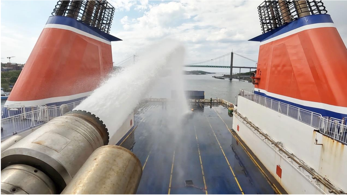
Figure 9. Photo from the perspective of the autonomous fire monitor suppressing one of twelve fires located in twelve random positions on the weather deck during the demonstration onboard the Stena Scandinavica.
