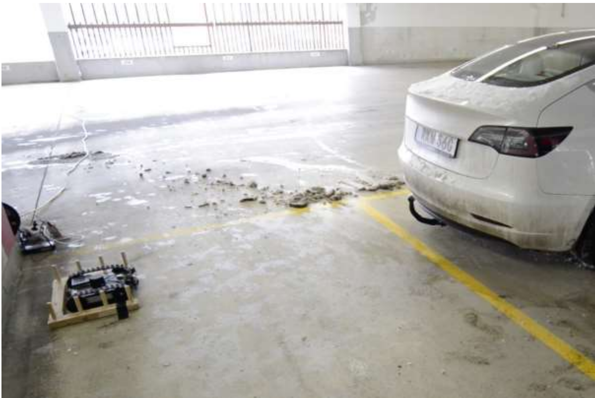
Figure 27. Test setup for test of license plate readout in relevant environment.
