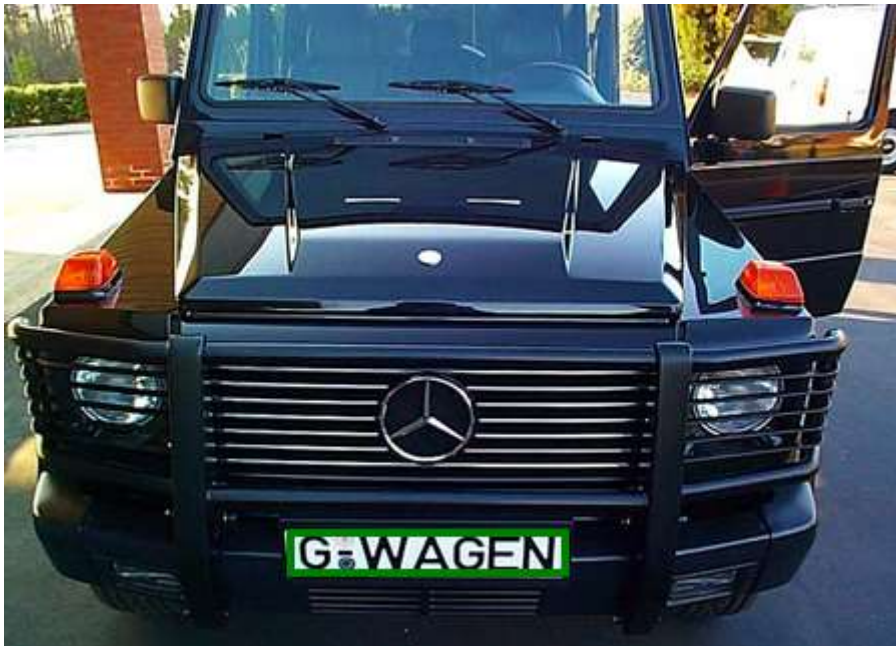
Figure 23. Correctly detected, but incorrectly classified vehicle by OpenALPR. Image modified from [2].
