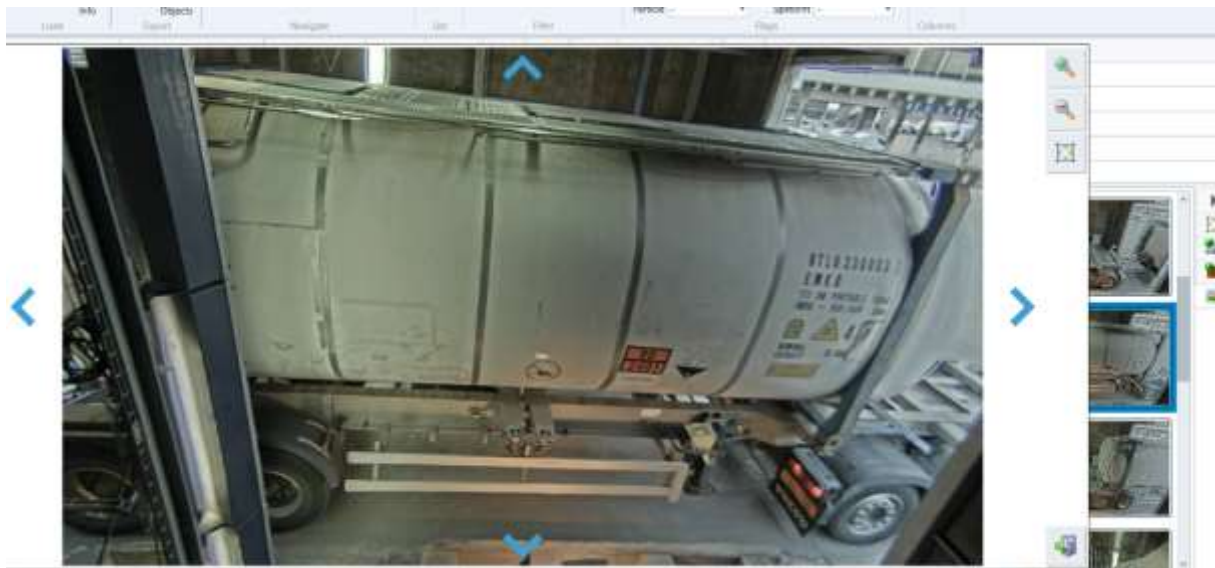
Figure 20 ADR/DG placard visible via CCTV.
