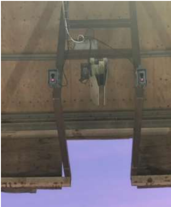
Figure 8 Front LPR and ANPR readers on each side of the LiDAR. (STL)
