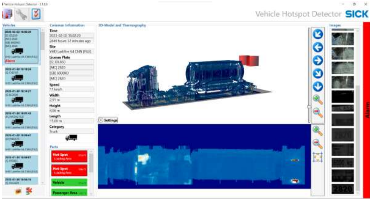
Figure 17 Overheated brakes on trailer with ADR/DG goods.
