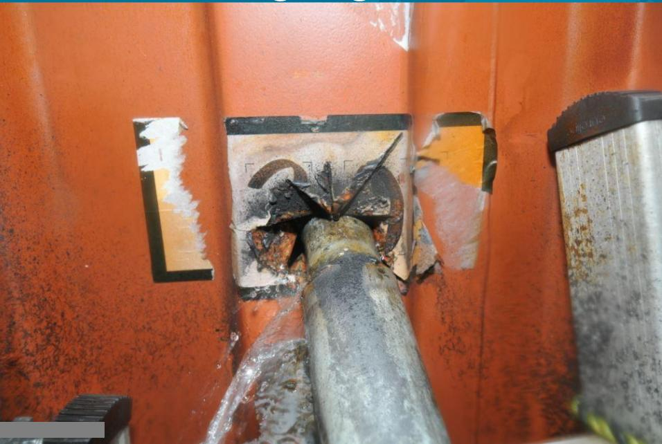
Burning material falling through the plywood floor
