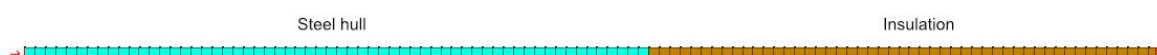
Figure 2. Image showing the FEM layout of the heat transfer model for a case with 6 mm thick steel hull (blue) and 5 mm of insulation (brown). The heated boundary is on the left of the image while the right hand boundary is to ambient (20°C) air.
