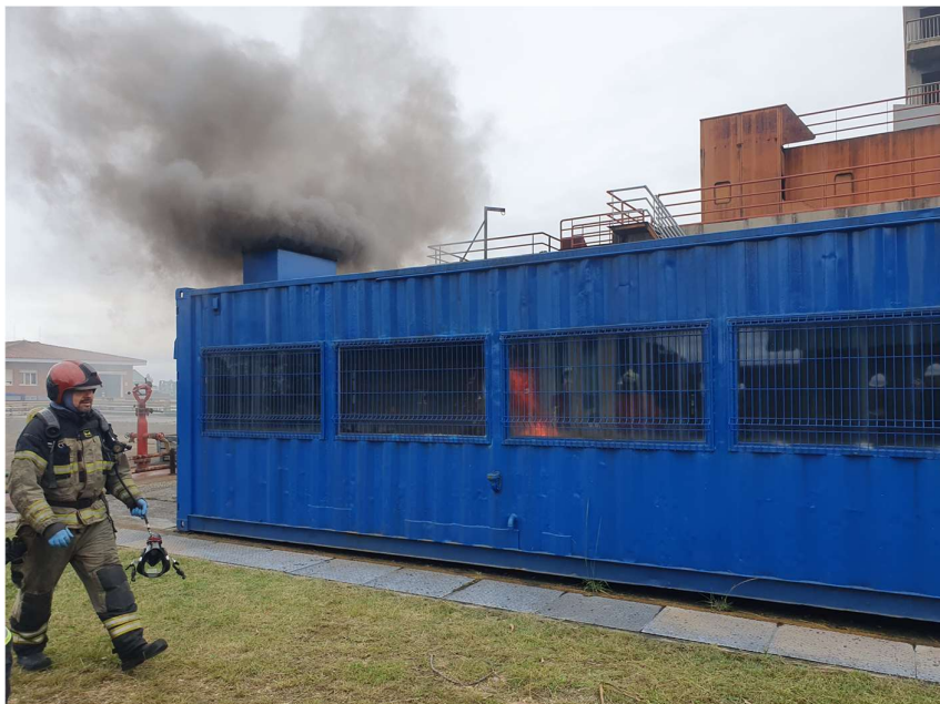
Figure 32. At this stage, the CO2 has been activated inside the container.
