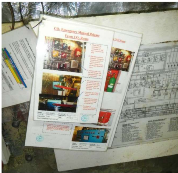
Figure 15. Image of two different operating instructions for the same CO 2 system that caused confusion in the 2018 Mignon fire.
