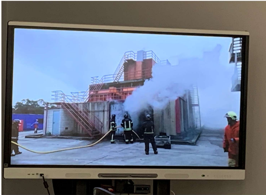
Figure 29. Manual firefighting after drencher deployment (view from the bridge).
