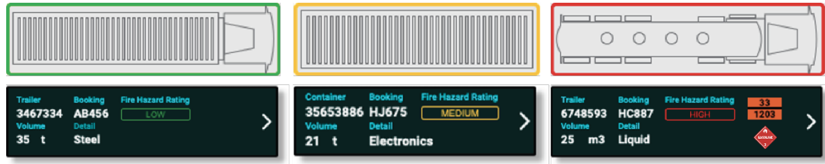
Figure 23. Representation of cargo on deck categorised in three fire hazard ratings (A) low, (B) medium, (C) High
