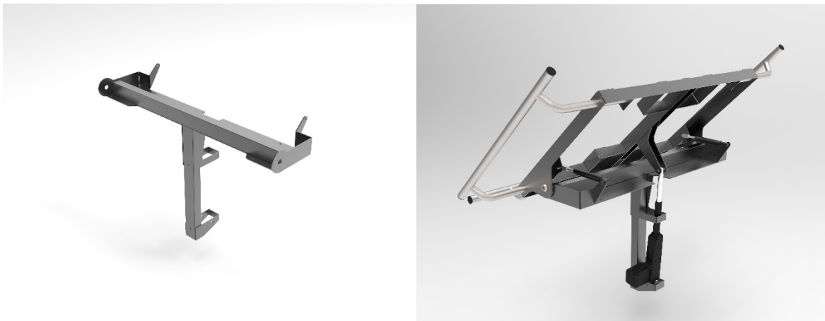
Figure 11. The T-frame on the left-hand side. On the right: Assembly of the tilt function involving the screen frame and the T-frame driven by an electric actuator and stabilised by two gas-springs.
