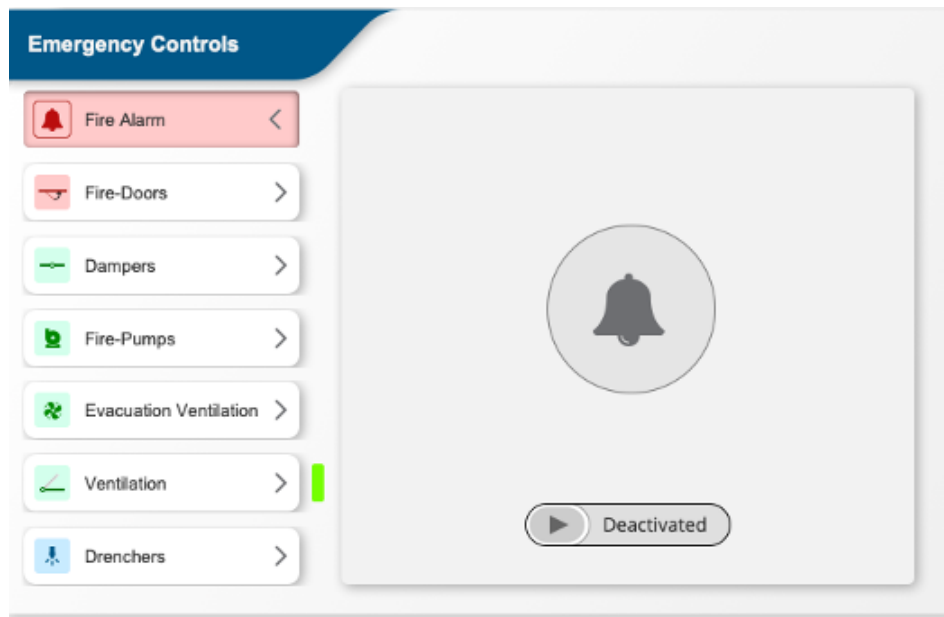
Figure 25. Emergency control with fire bells deactivated.
