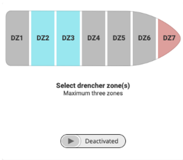
Figure 31. Emergency control to activate and deactivate the drencher system in different drencher zones.
