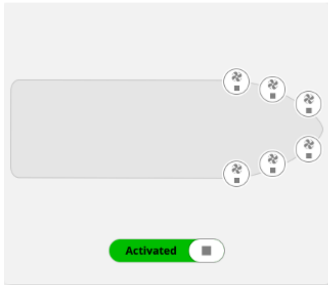
Figure 27. Emergency control to activate and deactivate the ventilation on deck.
