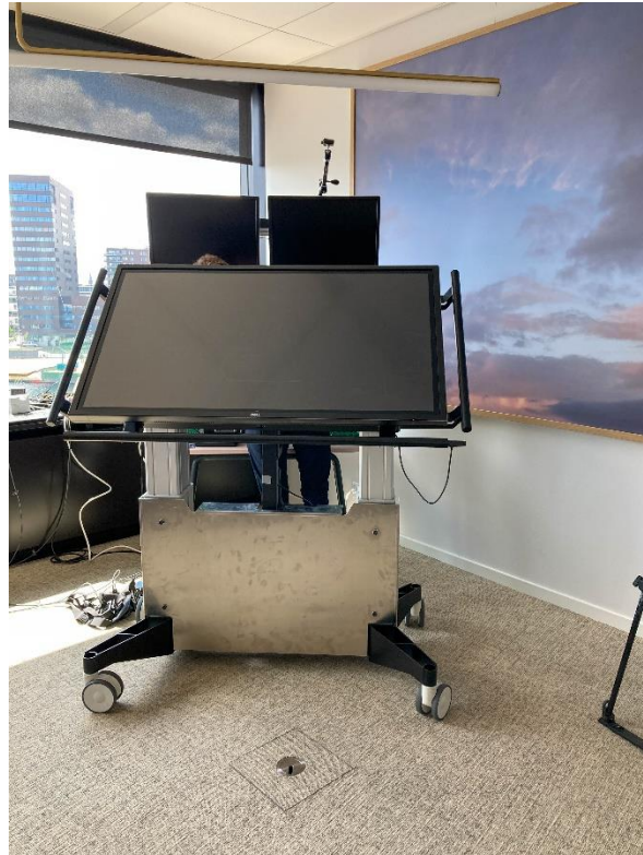
Figure 3 - The DFC demonstrator including the custom-built console, the 55" display as well as displays for CCTV and external drone
