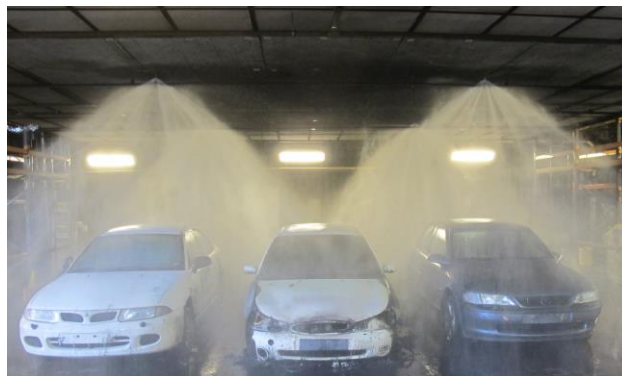
Figure 32. The discharge of water from automatic sprinklers (in another project than LASH FIRE).
