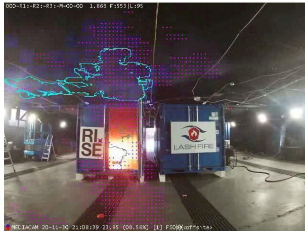
Figure 27. Image from a camera video clip that is post-processed by the video flame and smoke detection software. The flame inside the container is recognized by the software and marked with a grey outline and smoke is recognized and marked with a blue outline and purple dots.
