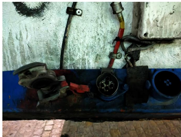
Figure 7. Faulty and dirty electrical connections on reefer.
