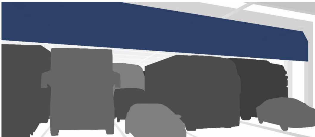
Figure 39. Solid curtain, vertical mounting, partly rolled down to top of high cargo/trucks.
