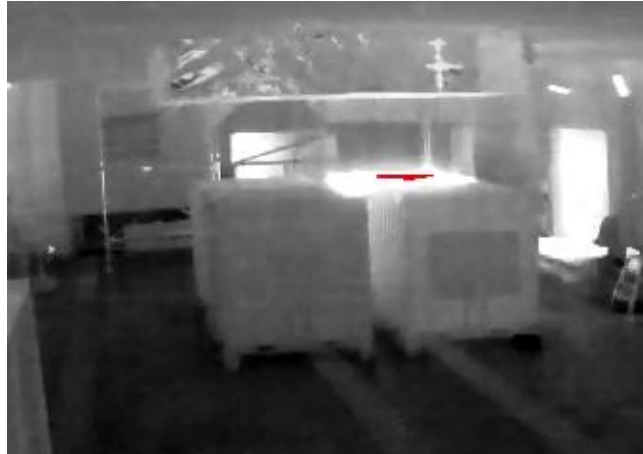
Figure 30. Example of how a visual confirmation could be obtained regarding a fire inside a closed container that using an IR thermal camera during a lab-scale test. This image is captured by the IR camera, showing that the roof of the container is hot as it is marked with a red colour, denoting high temperatures. The fire was not detected by any of the flame detectors as there were no visible flames outside the container.
