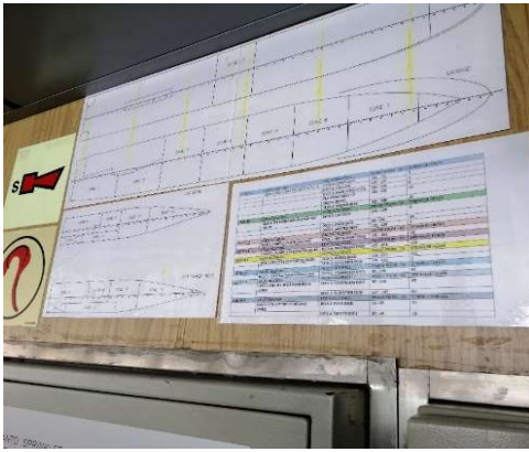
Figure 8. An example of a list of fire detectors positions and of information provided by the fire alarm panel
