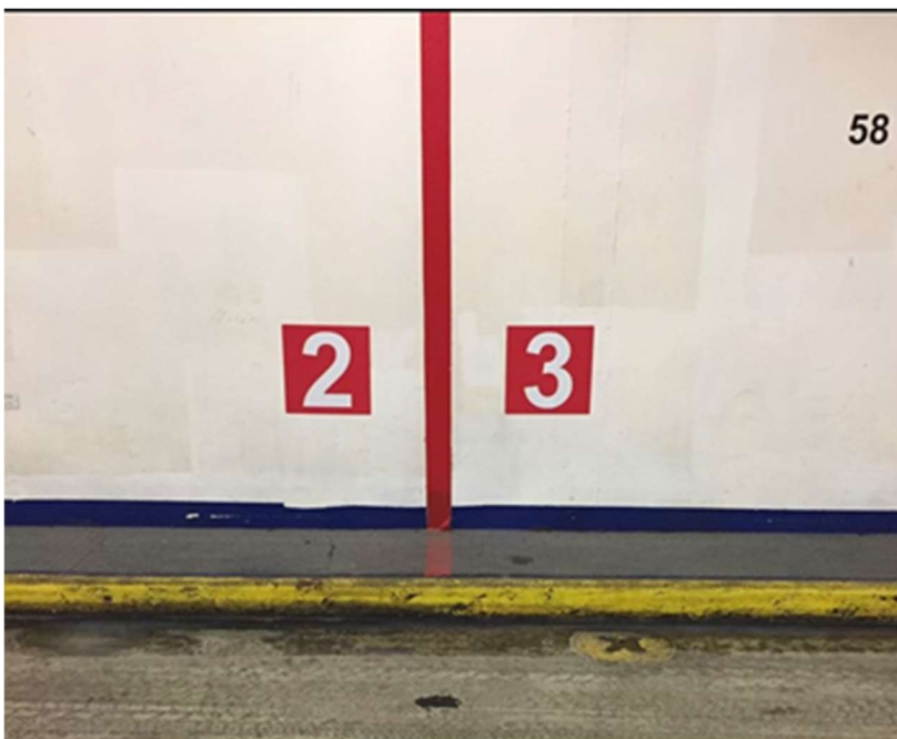
Figure 9. Drencher zone and frame markings on Stena Saga, realized with prefabricated “paint patterns” from supplier.
