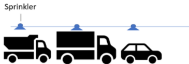
Figure 6: Drencher spray obstructed by cargo (Bram, Millgård, & Degerman, 2019).
