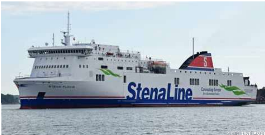
The Visentini Class ships operated by Stena were modified after the NORMAN ATLANTIC accident with a number of side openings closed to better safeguard LSAs as evidenced on STENA FLAVIA.
